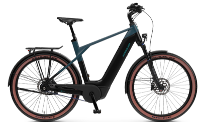
Vitality Eco 10 ..... 23 Shimano Nexus 5-Gang Freilauf / Bosch Performance Line CX / 750Wh / Disc / Gates
